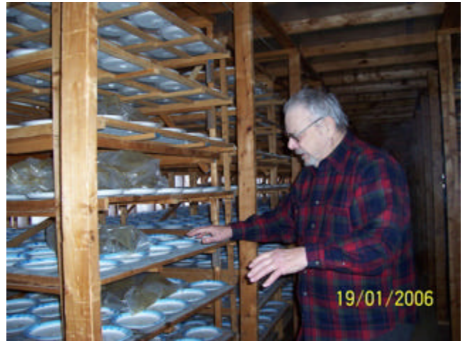
Mr. Butler showing the evaporation trays for the puréed clam viscera used in plant fertilizer. See "Peninsula Master Gardener News" for related article.
